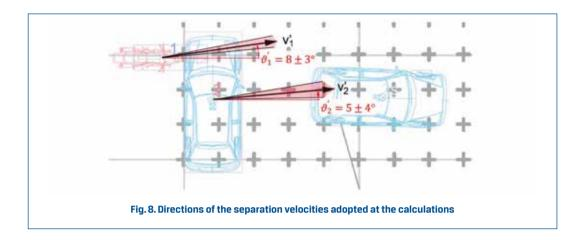
The mass of the test dummy representing the motorcyclist was  $m_0 = 82$  kg. After the motorcycle impact against the car, the dummy flew over the car bonnet without touching it; therefore, based on Priester's suggestions [18], a single combined value of the reduced mass of the motorcycle together with the motorcyclist, equal to  $m_j \approx m_{\gamma} + 0.3 \cdot m_0 = 207$  kg ( $\pm \Delta m_1 = 30$  kg) was assumed for the calculations where the momentum conservation principle was employed.
