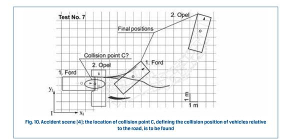
Let us use a mathematical model similar to that applied to the work described in publication [24]. The collision point is a selected point C situated on the tangential plane of the vehicles brought to contact with each other in accordance with the vehicle deformations. Since the position of this point in relation to both of the vehicles is constant, the calculation of its coordinates will in effect be the determining of the collision point.
