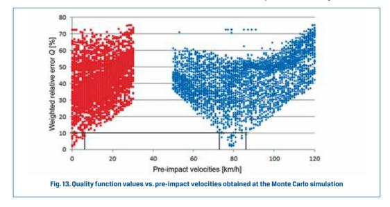
The fact that the expected value of the velocity of vehicle 1 determined from classical accident reconstruction calculations (86.8 km/h, see sub-item 3.1) was closer to the actual value (87.7 km/h) than that calculated with the use of the PC-Crash program (79.0 km/h) was pure chance. The simulations, which are virtual experiments, offer an incomparably more comprehensive view of the influence of different parameters than the simple momentum equations and McHenry formulas do.
