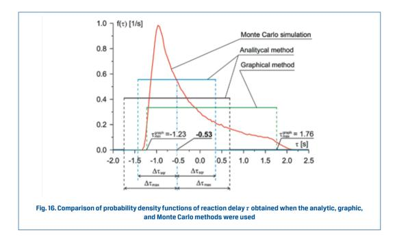
The uncertainty ranges determined with the use of the graphical and Monte Carlo methods practically coincide with each other and, in the nature of things, cover the whole span of the results possible. However, a good point of the Monte Carlo method is the fact that it additionally makes it possible to prepare the results in a form suitable for statistical processing.
