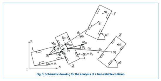
In the analysis, the notation as shown below has been adopted. Firstly, a symbol without an additional superscript (e.g.  $v_{.}$ ) relates to the pre-impact state; the sign "prime" (as in
